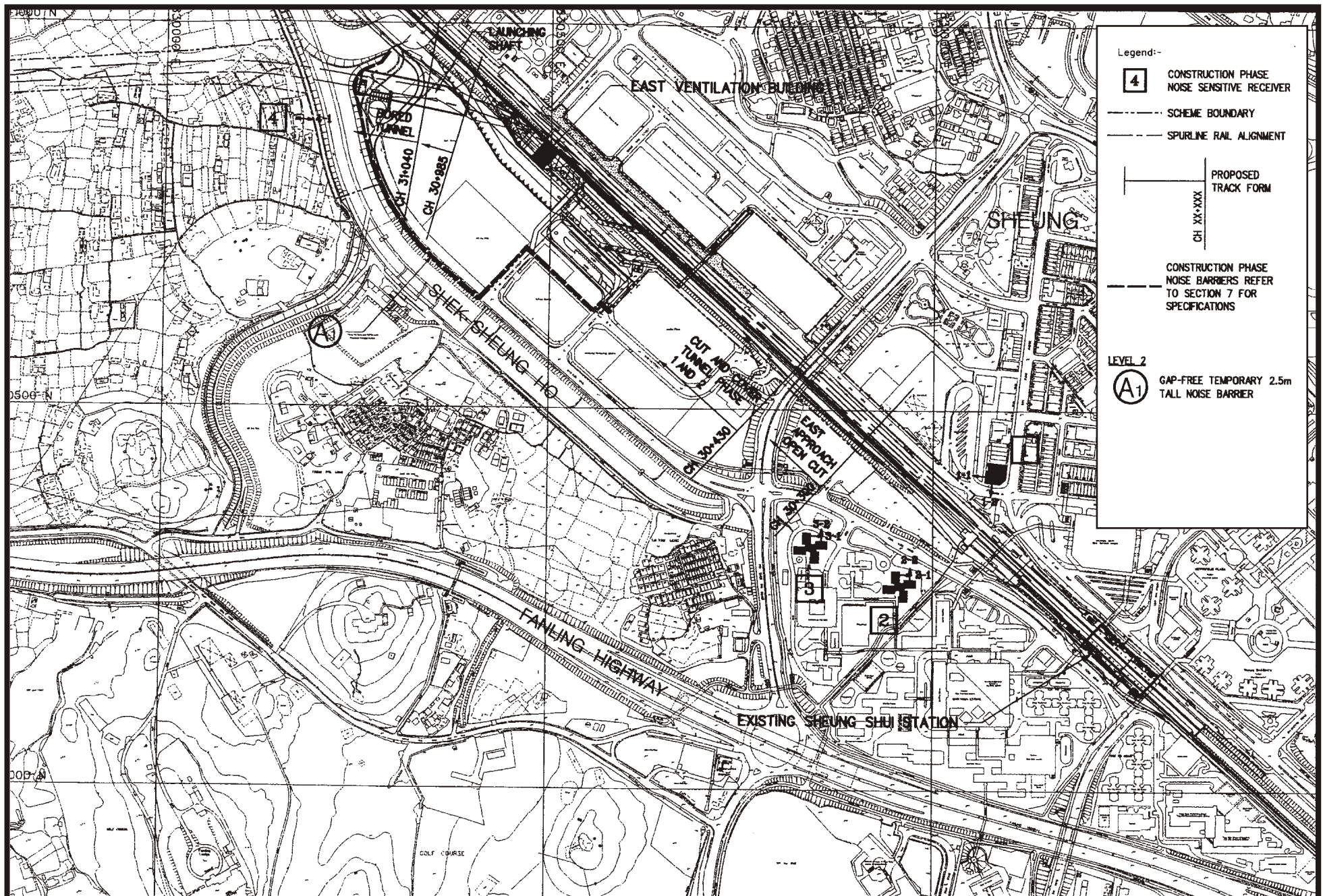
Figure 9a - Locations of Construction Phase Noise Barriers as described in Condition 3.25 of the Permit 圖九a - 條例3.25 所指消除建築工程噪音之隔音屏障位置 Reproduced from Drawing No. 7.1 (Sheet 1 of 5)(Volume 5 of 5) of the EIA Report (Register number AEIAR-
