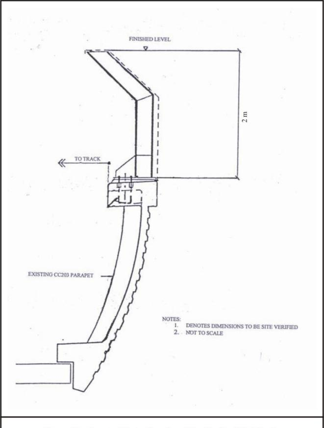
Figure 15 - Cranked Noise Barrier at the Tin Shui Wai Station
