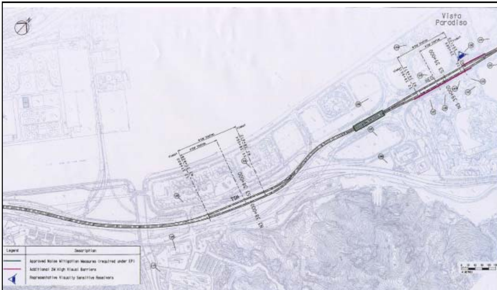
Figure 28 Locations of Additional 2m High Visual Barriers (Extracted from the Application VEP-157/2004)
