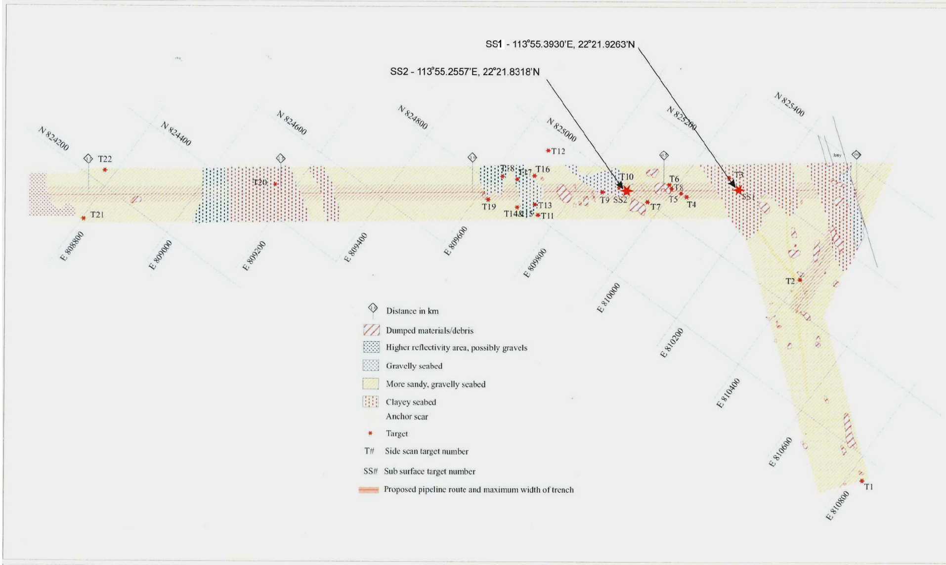
Figure 3: Positions of Sub-seabed Anomalies at SS1 and SS2 (Reproduced based on Figure 9.10 in EIA Report)
