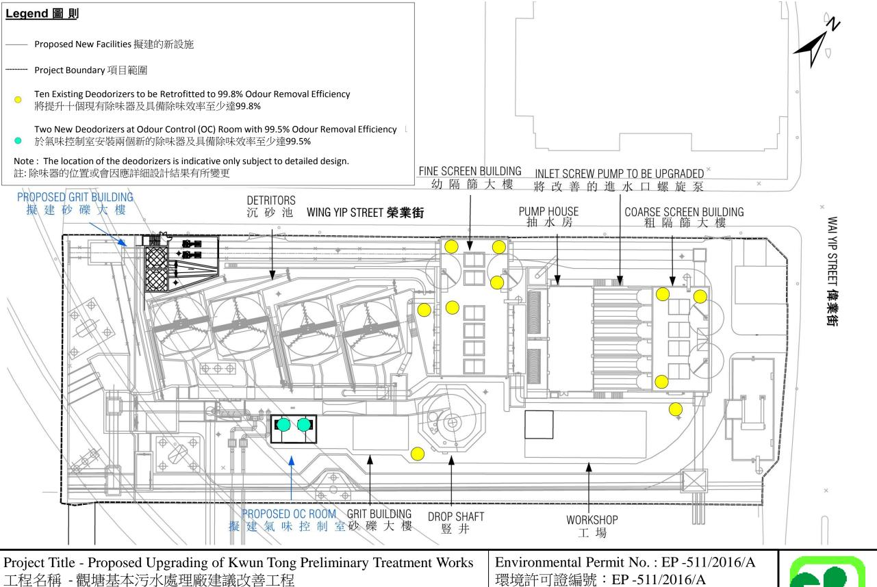
Figure 2 - Layout of the Upgraded Kwun Tong Preliminary Treatment Works and Location of Deodorizers 圖二 - 改善後的觀塘基本污水處理廠平面圖和除味器的位置
