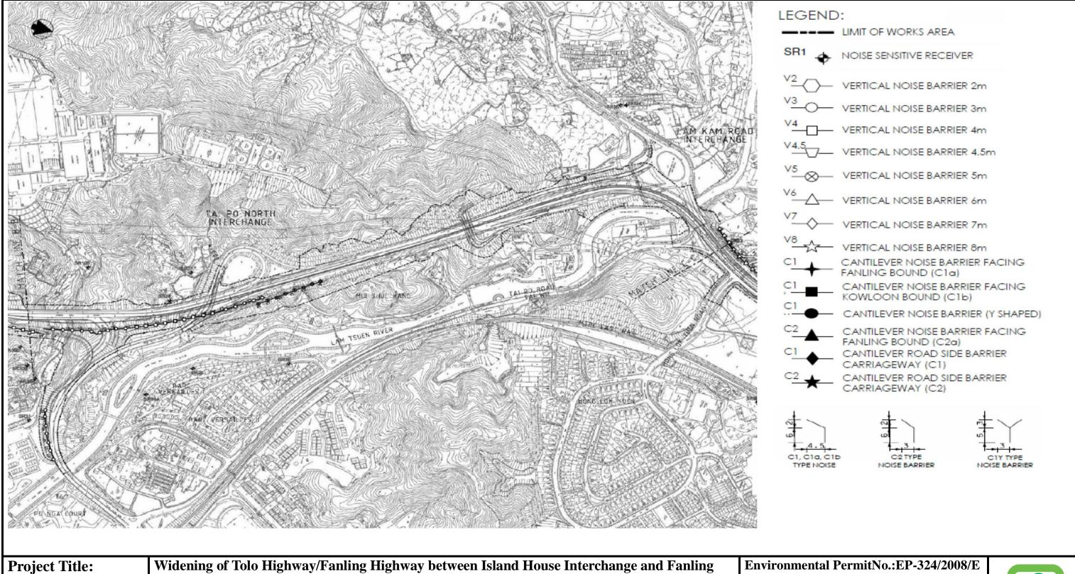
工程名稱: Figure 4c **Layout of Noise Barrier** 隔音屏障圖 圖四 c The figure was prepared based on Figure 4c of Application for Variation of Environmental Permits (No. VEP480/2015) 本圖是根據更改環境許可證申請(編號:VEP480/2015)的圖 4c 編制
