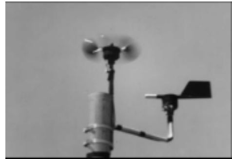
Anemometer and Wind Vane Mounted on top of Wind Monitoring Tower
