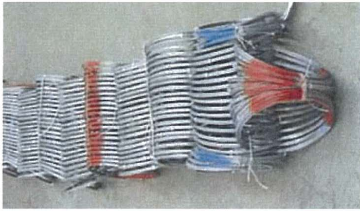
View of the flexible barrier prior to installation
