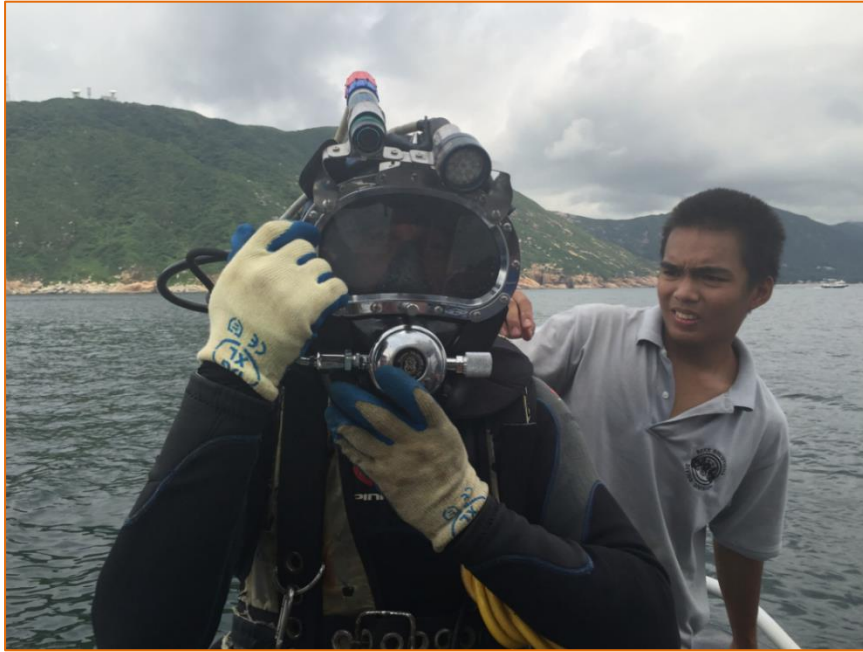
Figure D-7 Diver Wearing Helmed-mounted Video and Communications
