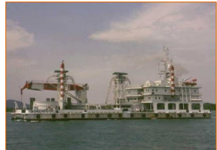
Typical Cable Installation Barge (Injector Tool)
