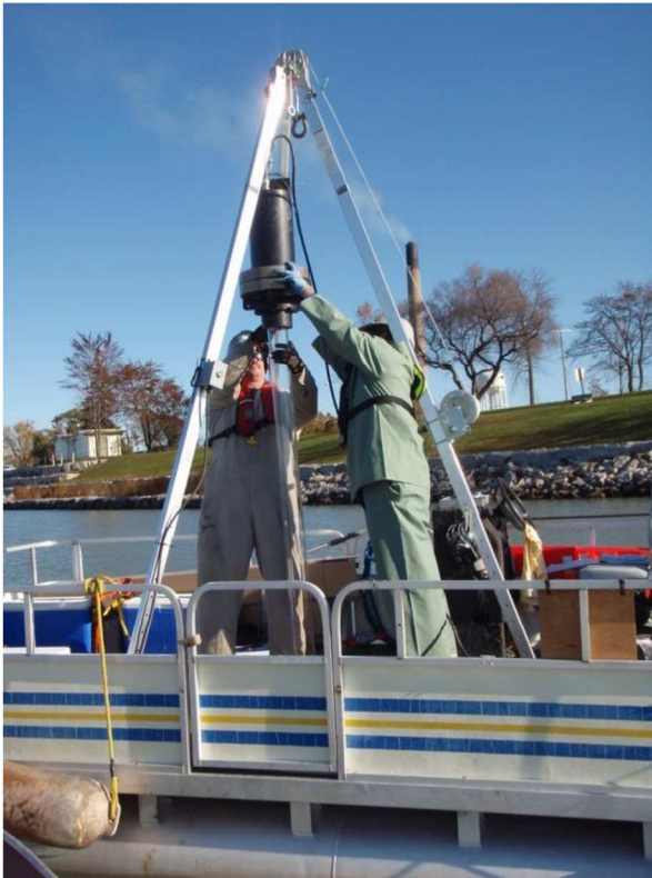
Plate 2 - Illustrative Photos of the Operation of a Typical Vibrocore sampling equipments
