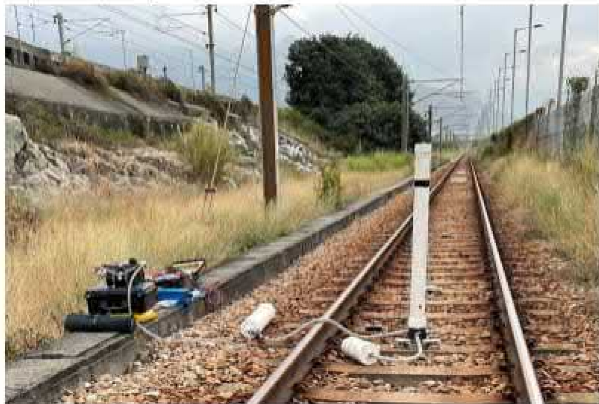
b) Photo of the Impact Hammer Setup at SHD Test Track
