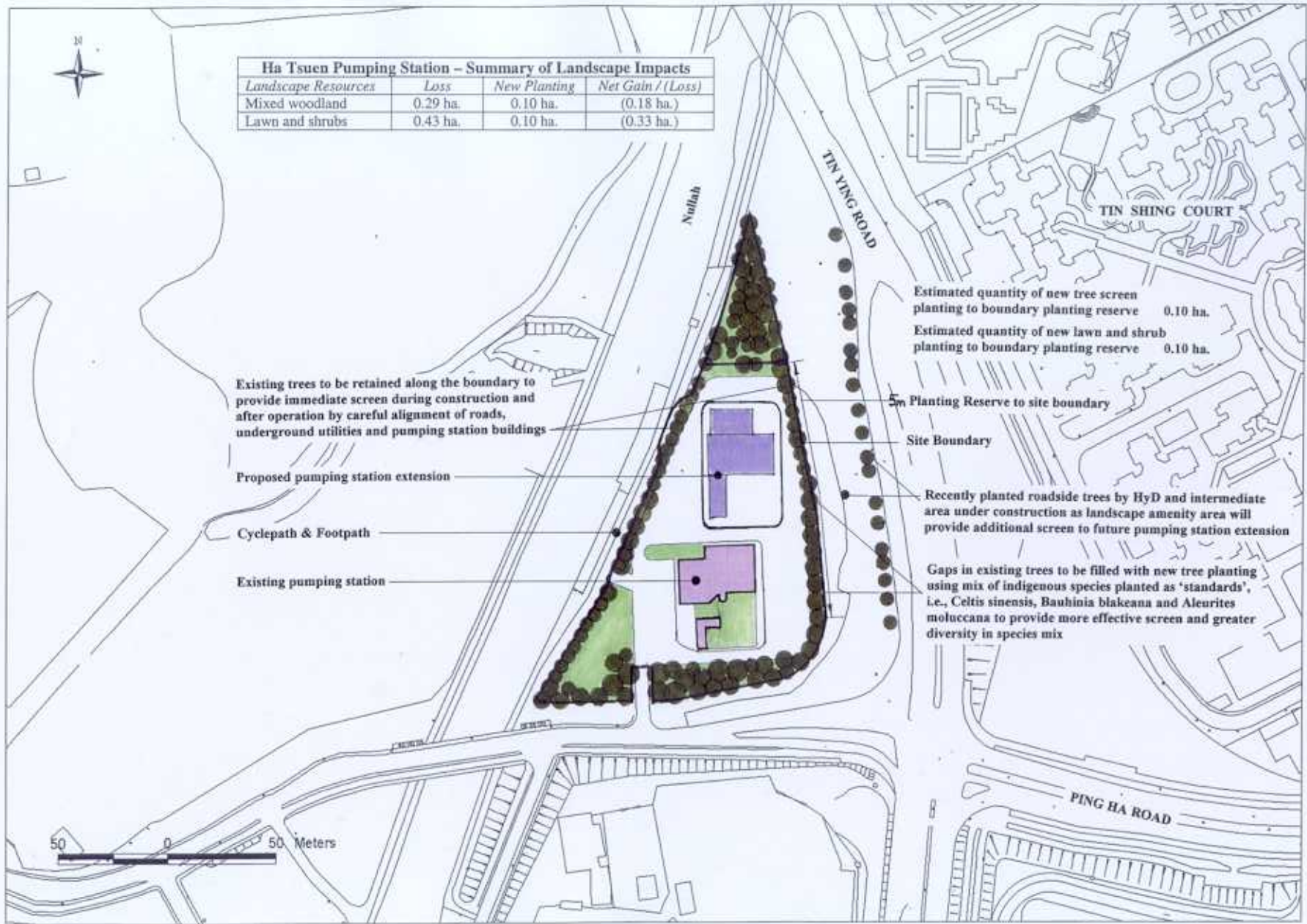
FIG. 11.7 HA TSUEN PUMPING STATION – MITIGATION PROPOSALS
