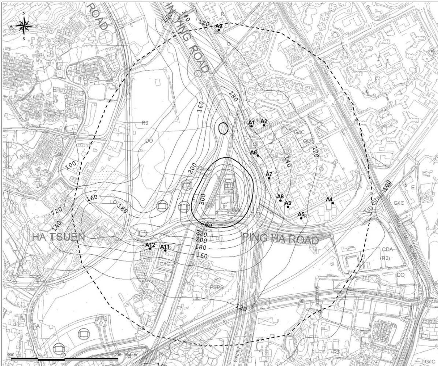
Figure 3.12 Predicted Worst-case Daily Average TSP Concentration Contours at 1.5m Above Ground for Unmitigated Scenario around the Proposed Expanded Ha Tsuen PS
