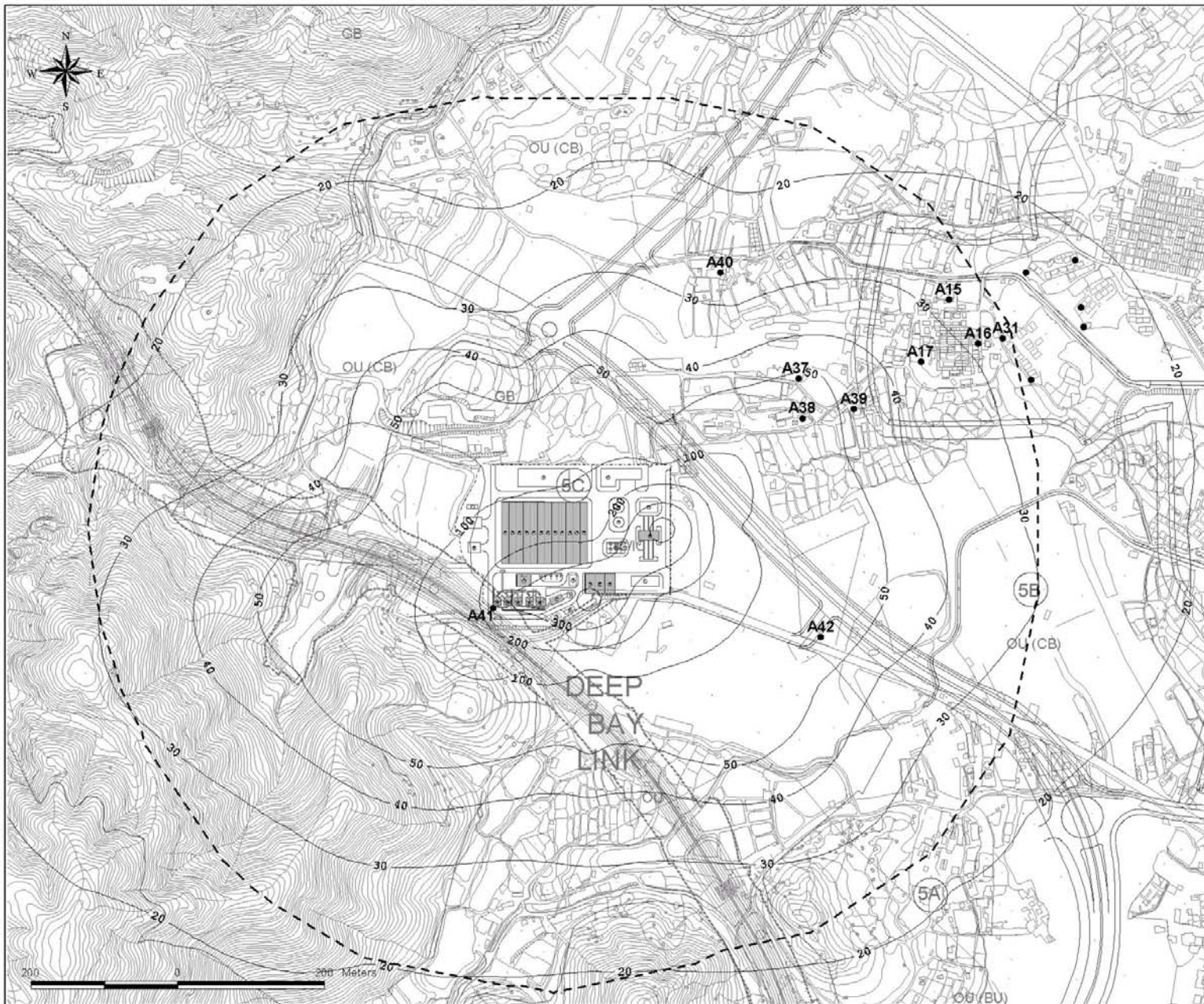
Figure 3.15 Predicted Worst-case 5-second Average Odour Levels at 1.5m above Ground for the Unmitigated Scenario around the Proposed Expanded and Upgraded San Wai STW
