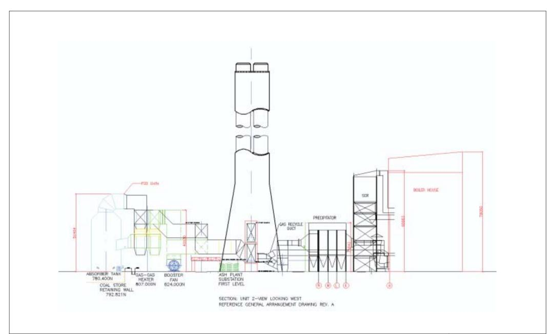
Figure 9.3 Cross Section of the Site showing the FGD and SCR Units in relation to the Existing Facilities - View Looking West
