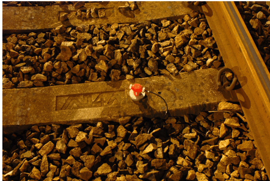
PHOTO 3 GEOPHONE MOUNTED ON THE SLEEPER 4.2m AWAY FROM THE IMPACT LOCATION
