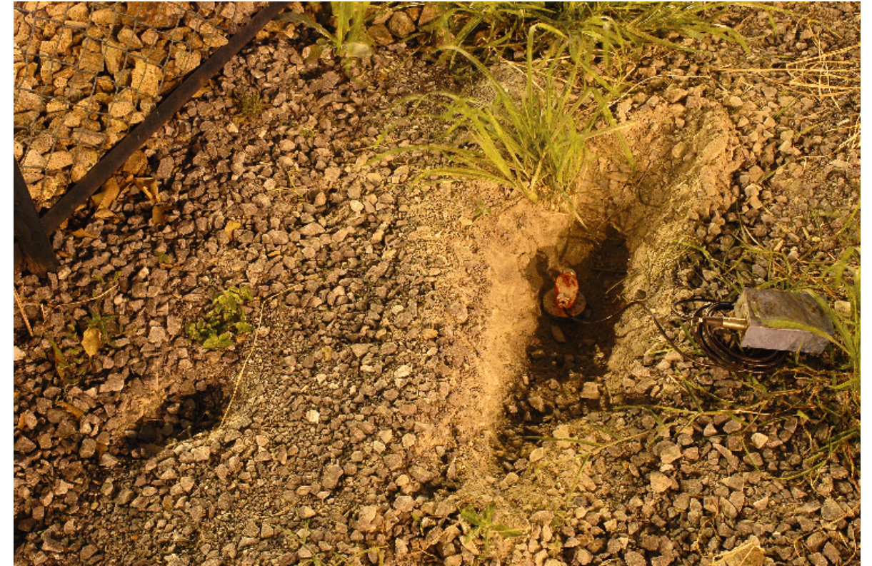
PHOTO 4 GEOPHONE MOUNTED ON THE SPIKE INSERTED INTO SOIL NEARBY THE TRACK
