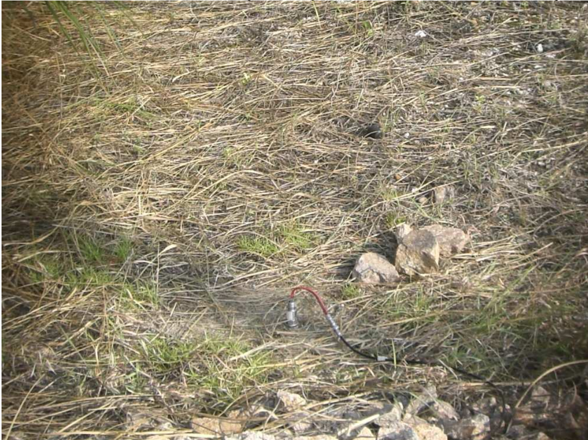
Photo 2: Vibration sensor mounted on top of a nail punched 150mm into soil at 12.5m from plain track
