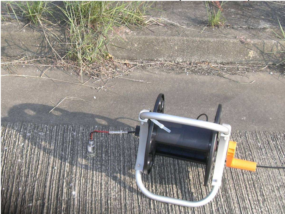
Photo 4: Vibration sensor mounted at concrete road surface by bee wax at 25m from plain track
