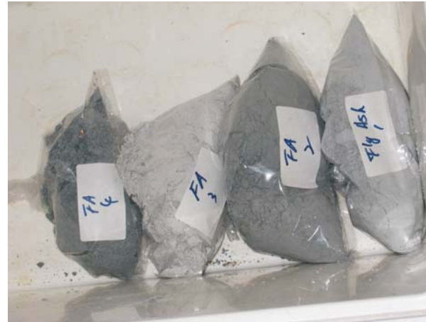
Samples were labelled and stored for delivery to laboratory testing (Fly Ash)
