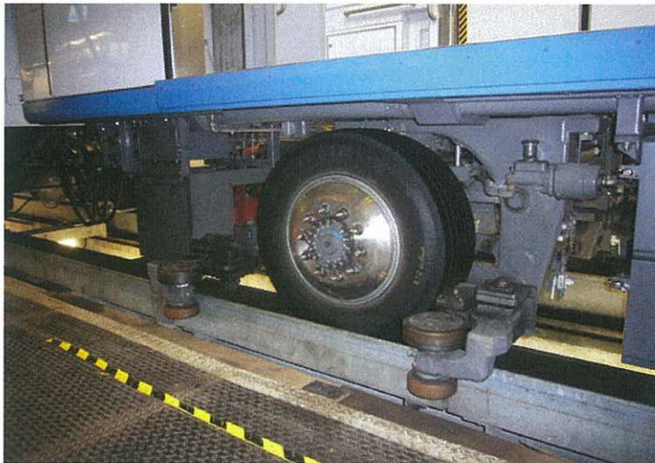
Existing APM - Inflated Tyres and Guide Wheels for APMs
