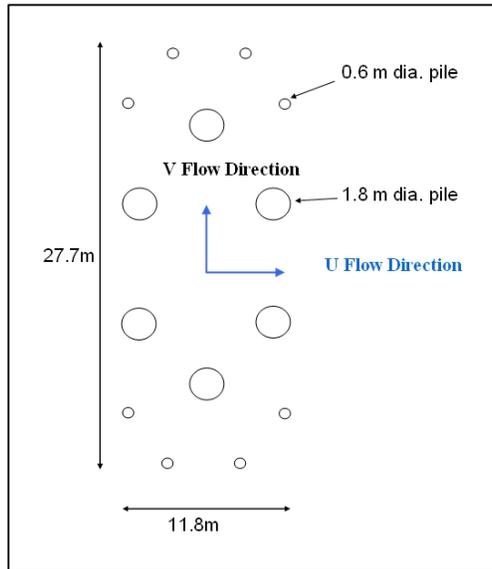
**Figure 1 TM-CLKL Bridge Pier Arrangement**
