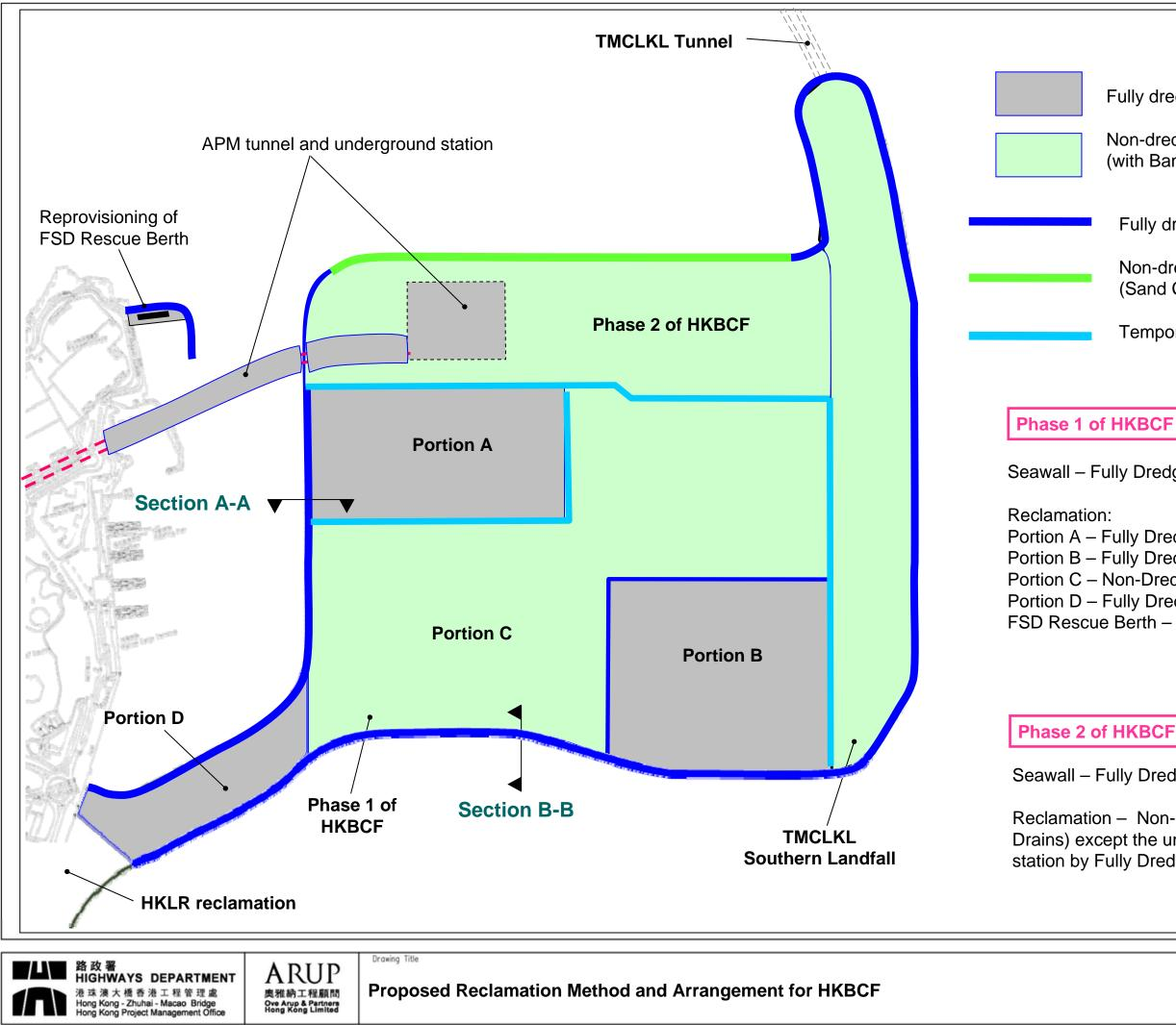
Fully dredged Non-dredged (with Band Drains) Fully dredged seawall Non-dredged seawall (Sand Compaction Pile - SCP) Temporary seawall Seawall - Fully Dredged Portion A – Fully Dredged Portion B – Fully Dredged Portion C – Non-Dredged (with band drains) Portion D – Fully Dredged FSD Rescue Berth – Fully Dredged
