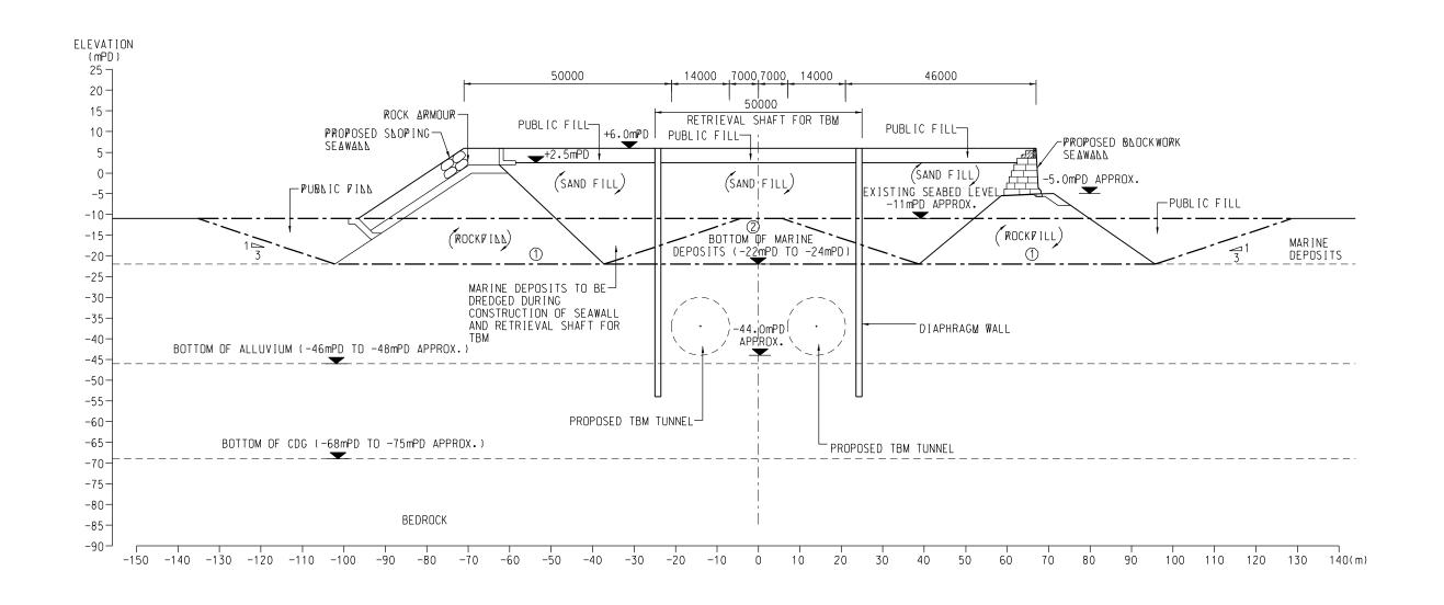
LEGEND: EXTENT OF MARINE DEPOSITS TO BE DREDGED 1 DREDGING DURING CONSTRUCTION OF SEAWALL DREDGING FOR CONSTRUCTION OF TBM SHAFT
