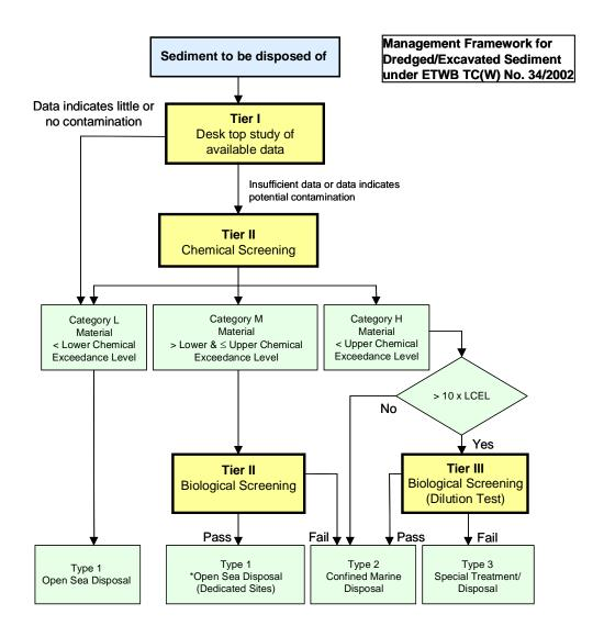
**Figure 6.3** Management Frameworks for Dredged/Excavated Sediment
