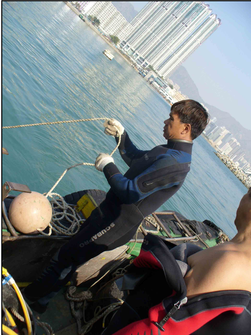
Figure 4.7: Diver positioning sinker to use as the centre point for the target search
