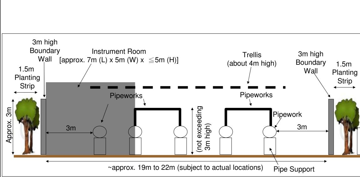
The proposed pigging station will be situated in a fenced-off area bound by solid boundary wall (3m height) on 4 sides. The covers an area of approximately 662 square metres. There will be an instrument room inside the proposed gas pigging static a simple structure with height not exceeding 5m after installation of some equipment on its top such as CCTV camera, air co and solar panels, etc. The instrument room itself is about 3m high only.
