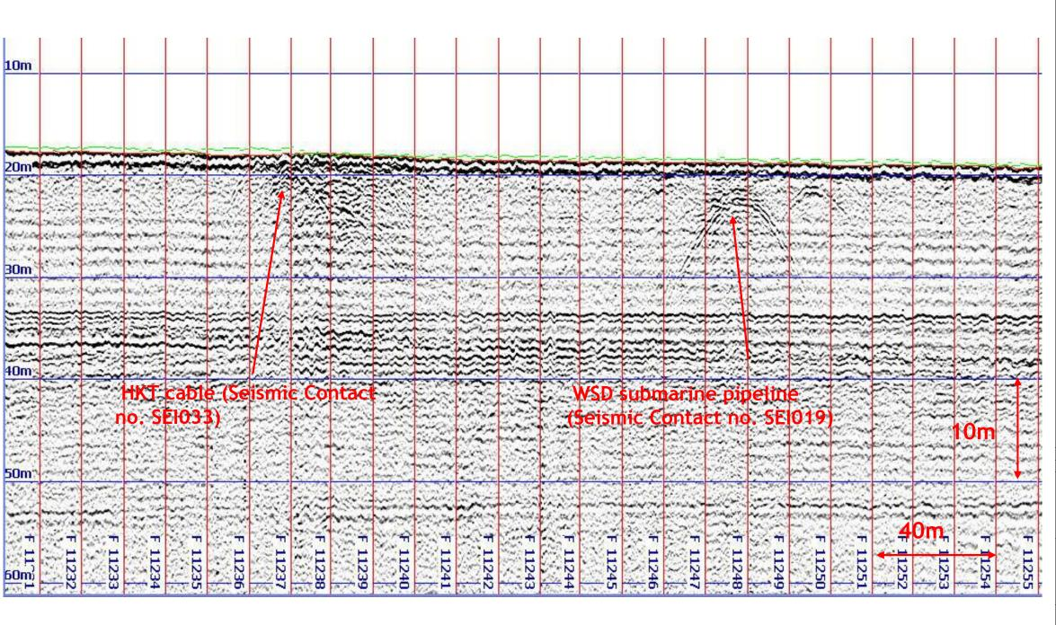
Figure 9.20: Seismic Data showing acoustic hyperbola associated with HKT buried cable and WSD pipeline.
