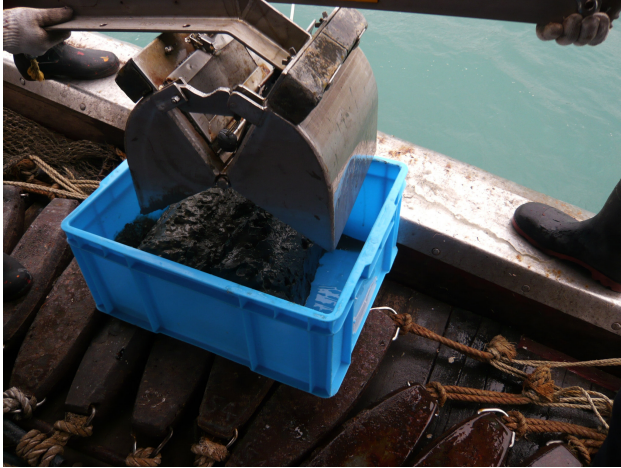
Plate 10. The grab in action at Station A.
