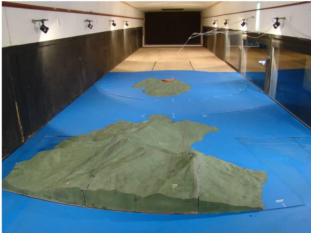
Figure 7. Photographs of the wind-tunnel configuration for the SKC site: a) 180 degree wind direction, downwind view; b) 180 degree wind direction, upwind view.
