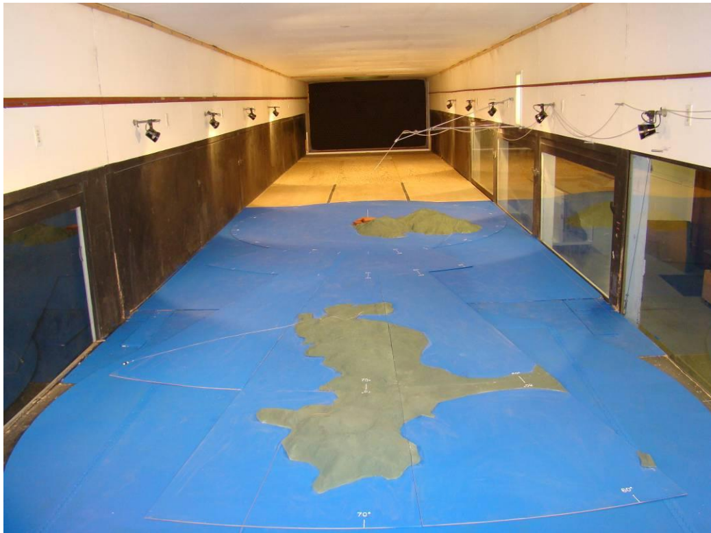
Figure 7. Photographs of the wind-tunnel configuration for the SKC site: c) 250 degree wind direction, downwind view; d) 250 degree wind direction, upwind view.
