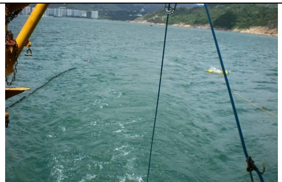
The EGS boomer and hydrophone were towed astern of the vessel for sub-bottom seismic profiling
