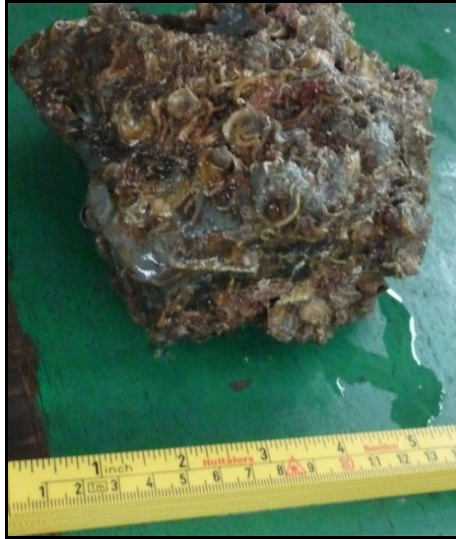
Figure 10: Modern building rubble retrieved at the location of SC003 and brought to the surface for validation.
