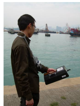
A sniffing team member was conducting H 2 S measurement on the site
