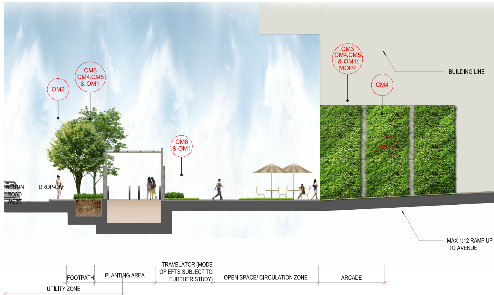
SECTION A - A (AUSTIN ROAD WEST) SCALE 1:150M @A3
