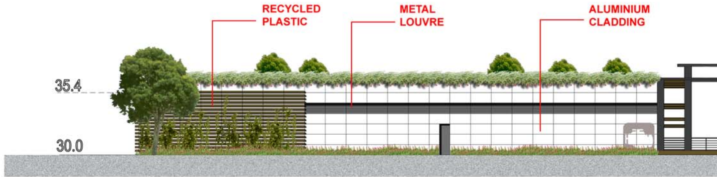
Transformer / pump station - East Elevation
