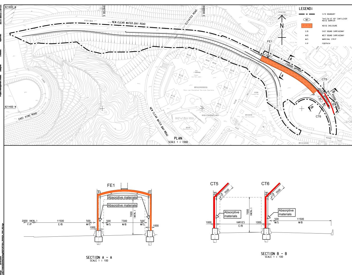
Note: The absorptive materials labels are for indicative purpose. Exact extent of the absorptive materials to be applied on the panel of the noise barriers or semi-enclosure are subject to be further designed.
