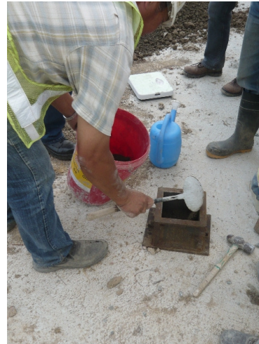
Photo 08 – Preparation of concrete cube.
