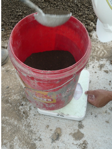
Photo 07 – The treated soil was weighed.
