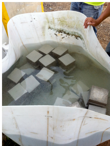
Photo 11 – Curing of concrete cube.
