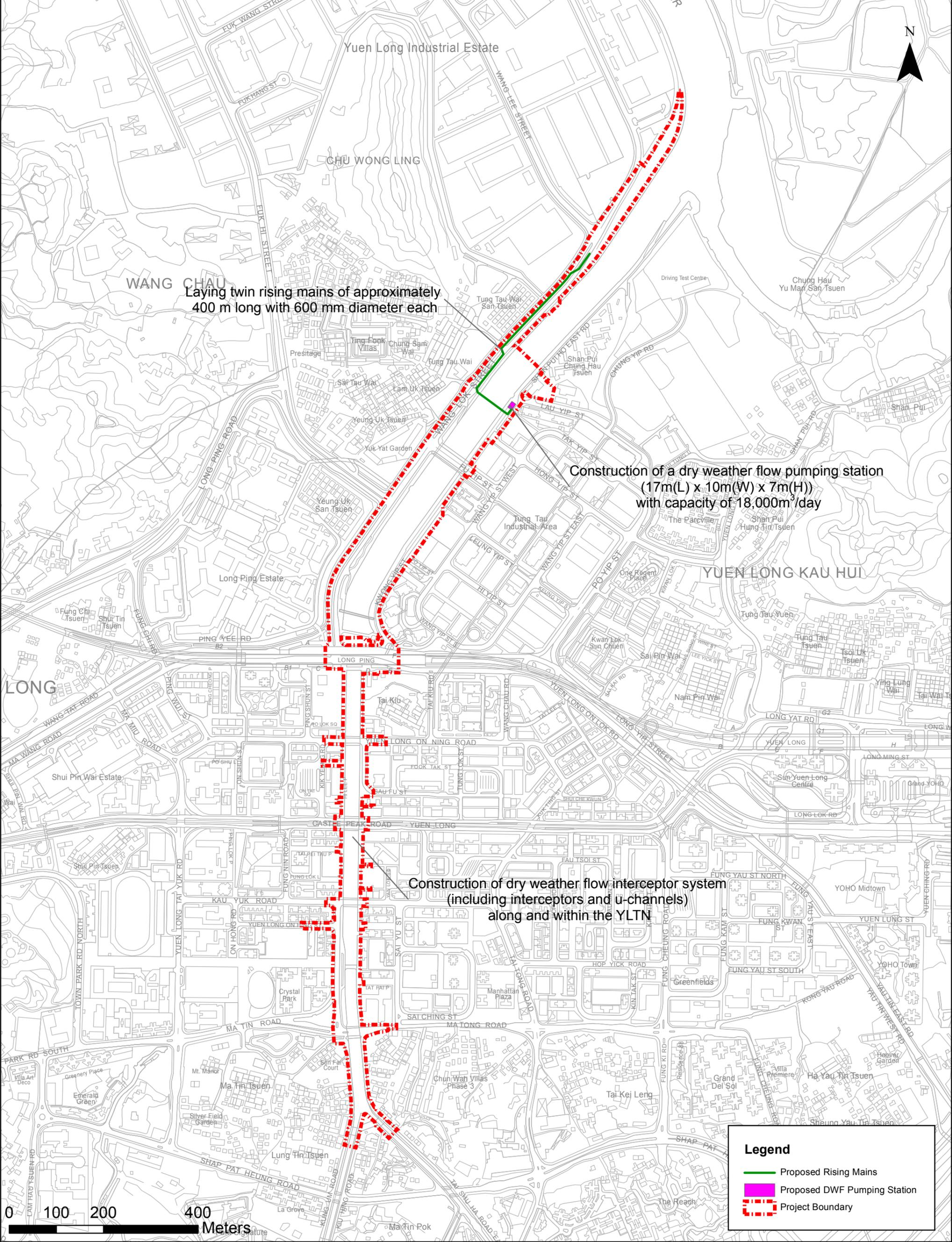
Laying twin rising mains of approximately 400 m long with 600 mm diameter each
