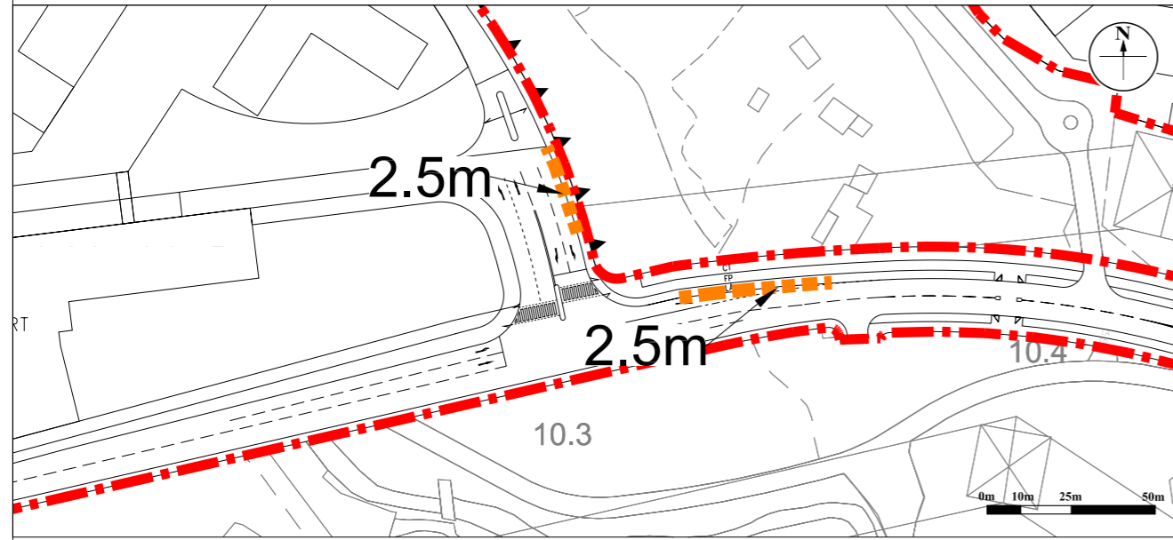
ADOPTED NOISE MITIGATION MEASURES IN CALINE4 MODEL AT HONG PO ROAD ACCESS ROAD
