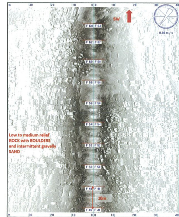
Figure 4 Side Scan Sonar data showing rocks and boulders in the south-western survey area
