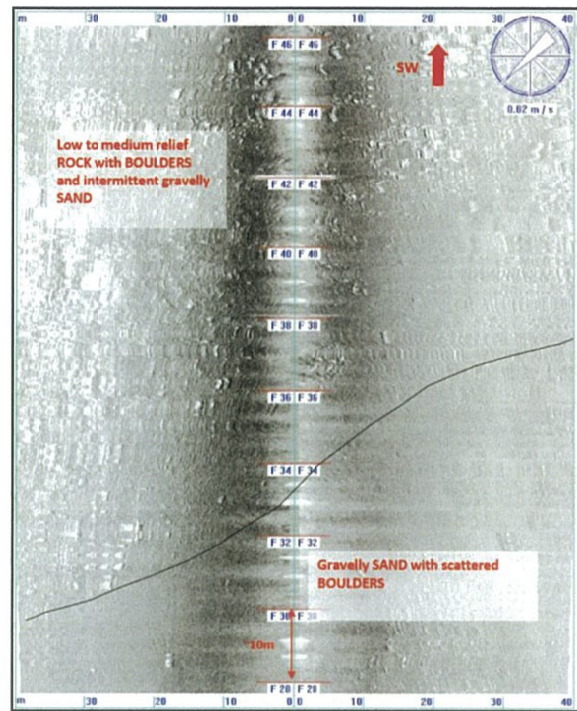
Figure 5 Side Scan Sonar data in the middle of the survey area
