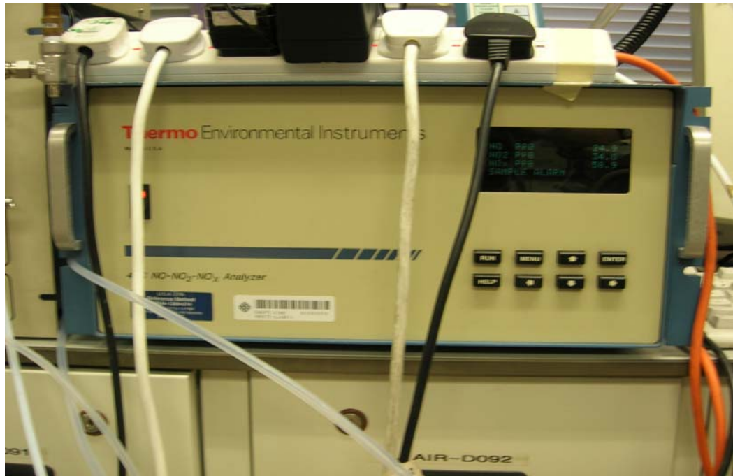
Fig.5. Chemiluminescence NO analyzer
