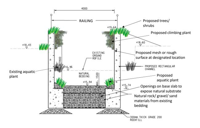
Figure 5.19 – Profiles of original watercourse and proposed green channel at Lin Fa Tei
