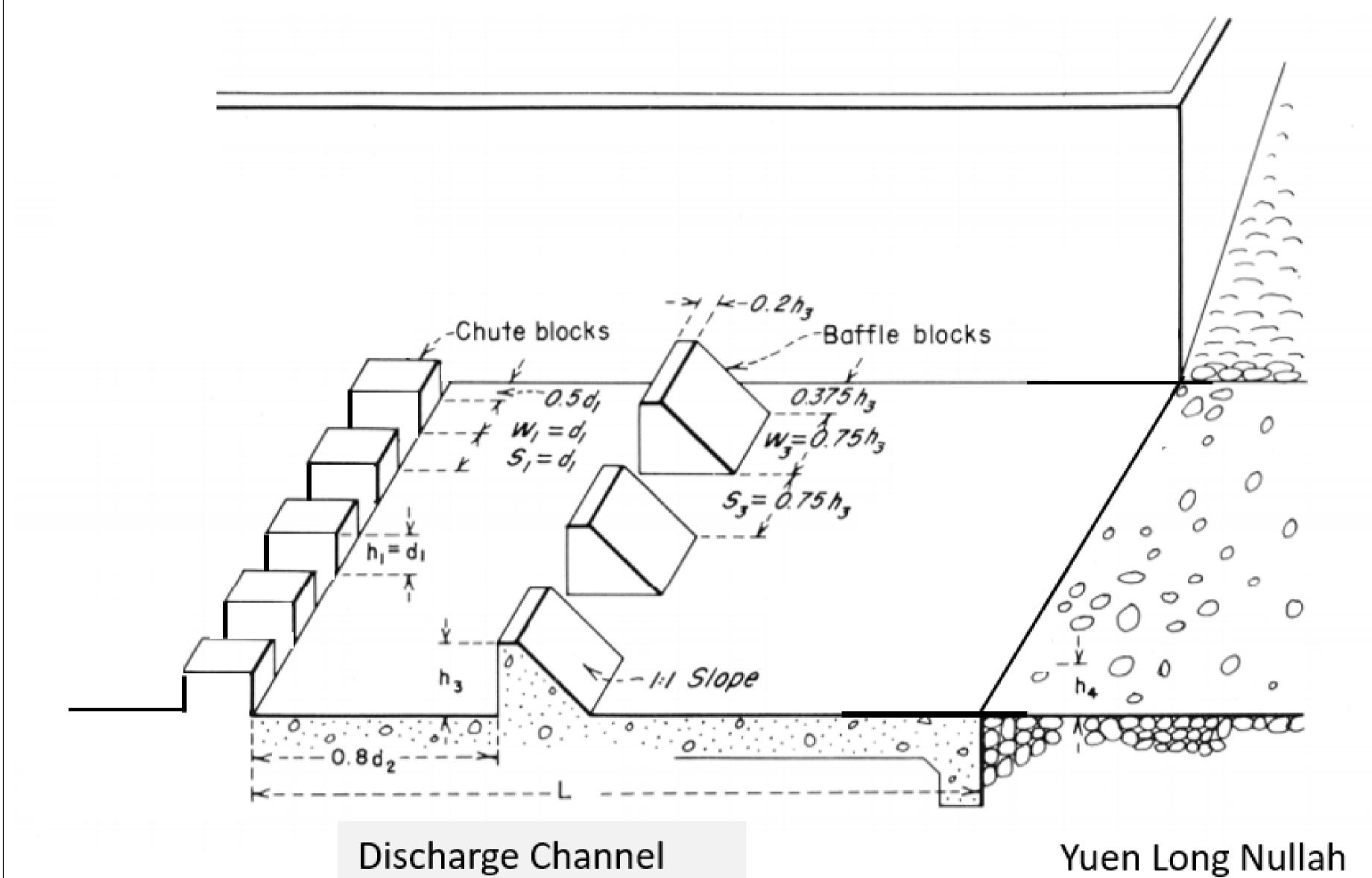
Examples of baffle blocks as energy dissipators in Hong Kong's drainage project
