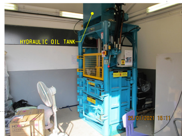
PHOTO 1022: HYDRAULIC WASTE BALER IN TUEN MUN COMMUNITY GREEN STATION (SITE TME-S1) (DATE TAKEN: 25 JANUARY 2021)
