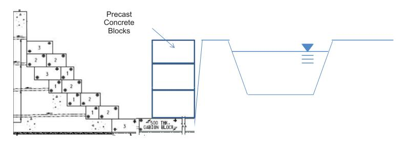
4. Divert the water flow from upstream to the constructed part of channel
