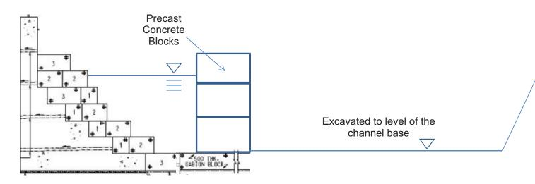
6.Construct channel bed and channel wall at the other side.
