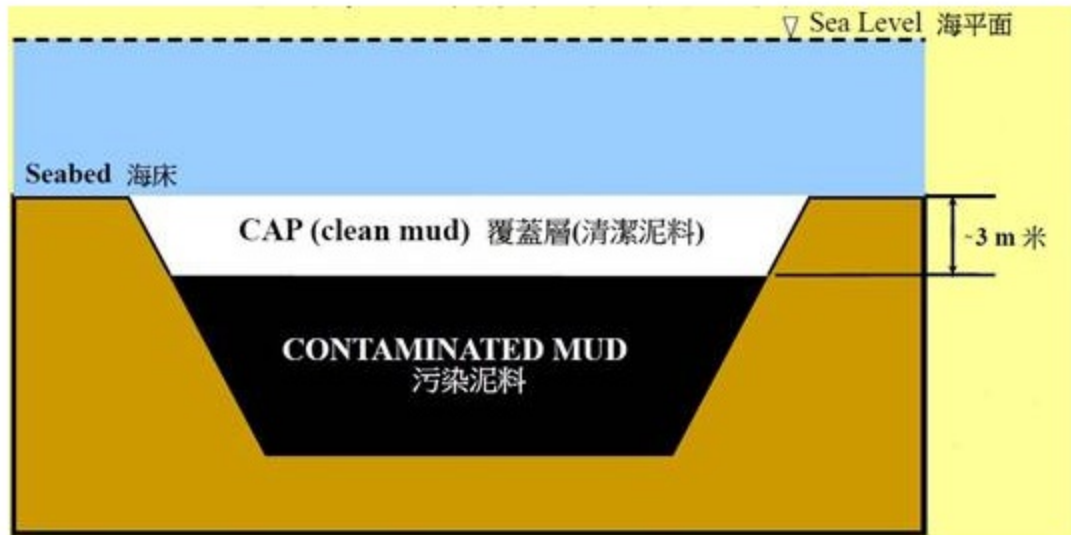
Figure 2.1 Typical Design of CAD Facility
