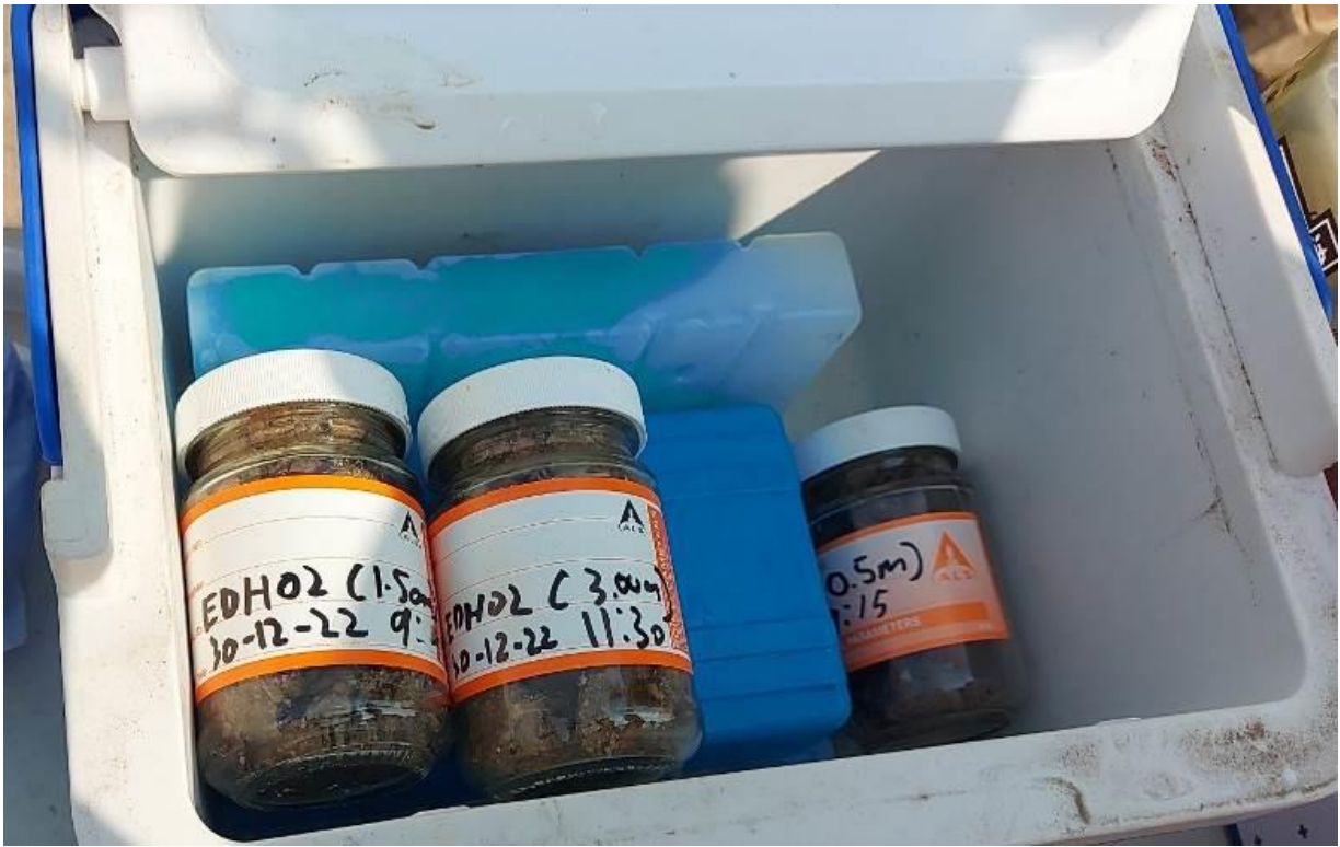
Photo 7: Sample container and cooler storage pending deliver to laboratory
