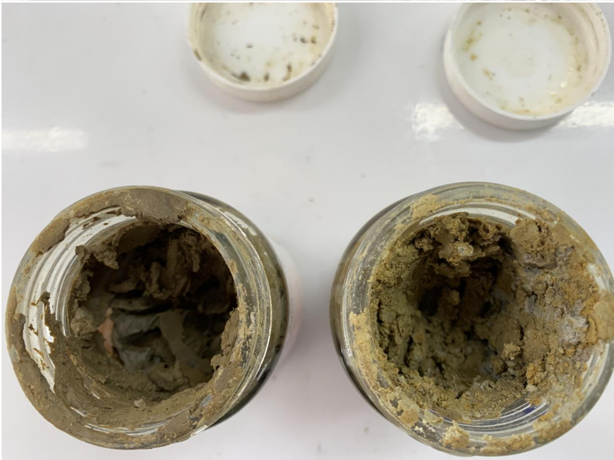
Photo 8: Photo of soil sample AEDH13 – 1.5m, primary sample is more clayey and brow (left), duplicate sample is more silty and with some grey colour (right)
