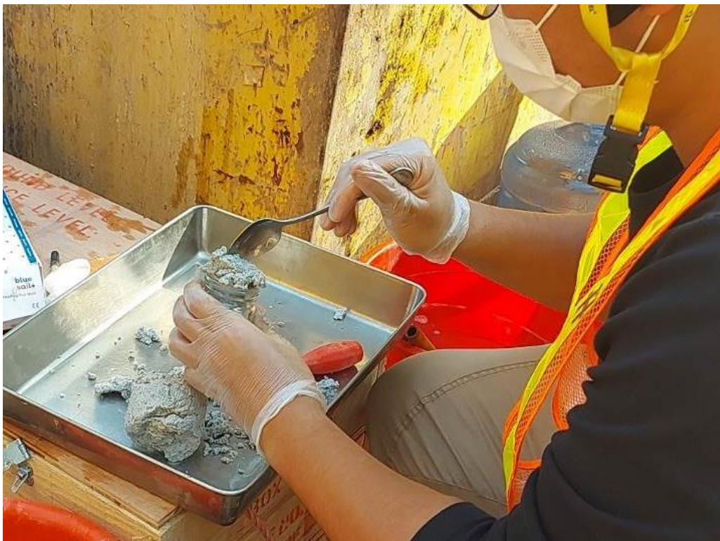
Photo 6: Transferring sample from U100 to soil container
