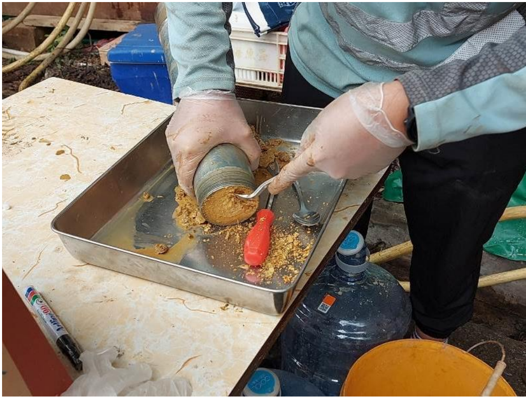
Photo 5: Transferring sample from U100 to soil container
