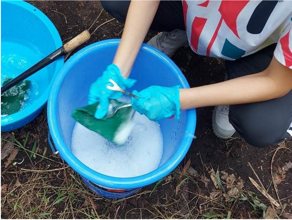
Photo 3: Decontamination of equipment between sampling events
