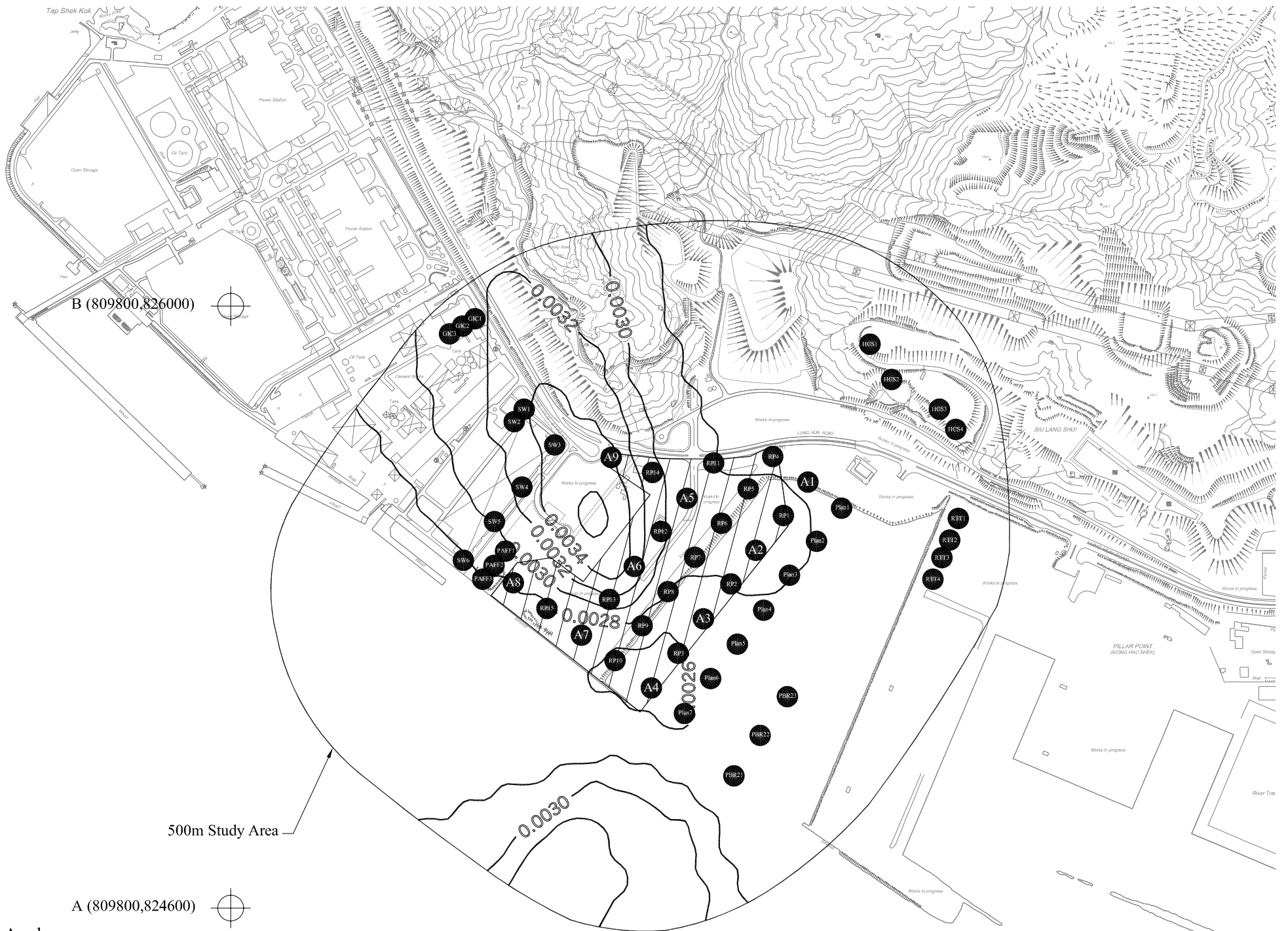
Figure 7-11 Cumulative 1-year Cd Concentration ( \mu\text{g}/\text{m}^3 ) at Ground Level emitted from Source Location A4 (Mitigated Scenario 2)
