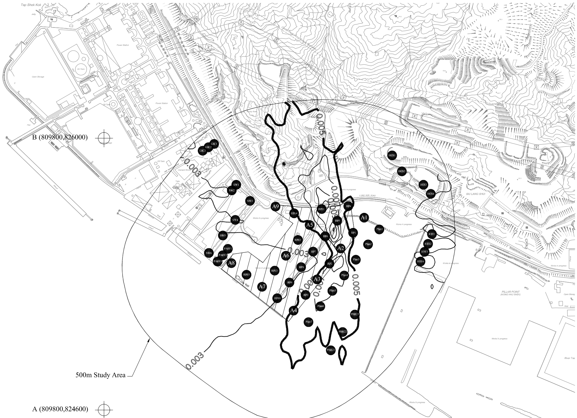
Scale: As shown Figure 7-I5 Cumulative 1-year Cd Concentration ( \mu\text{g}/\text{m}^3 ) at 61.5mPD emitted from Source Location A2 (Mitigated Scenario 2)
