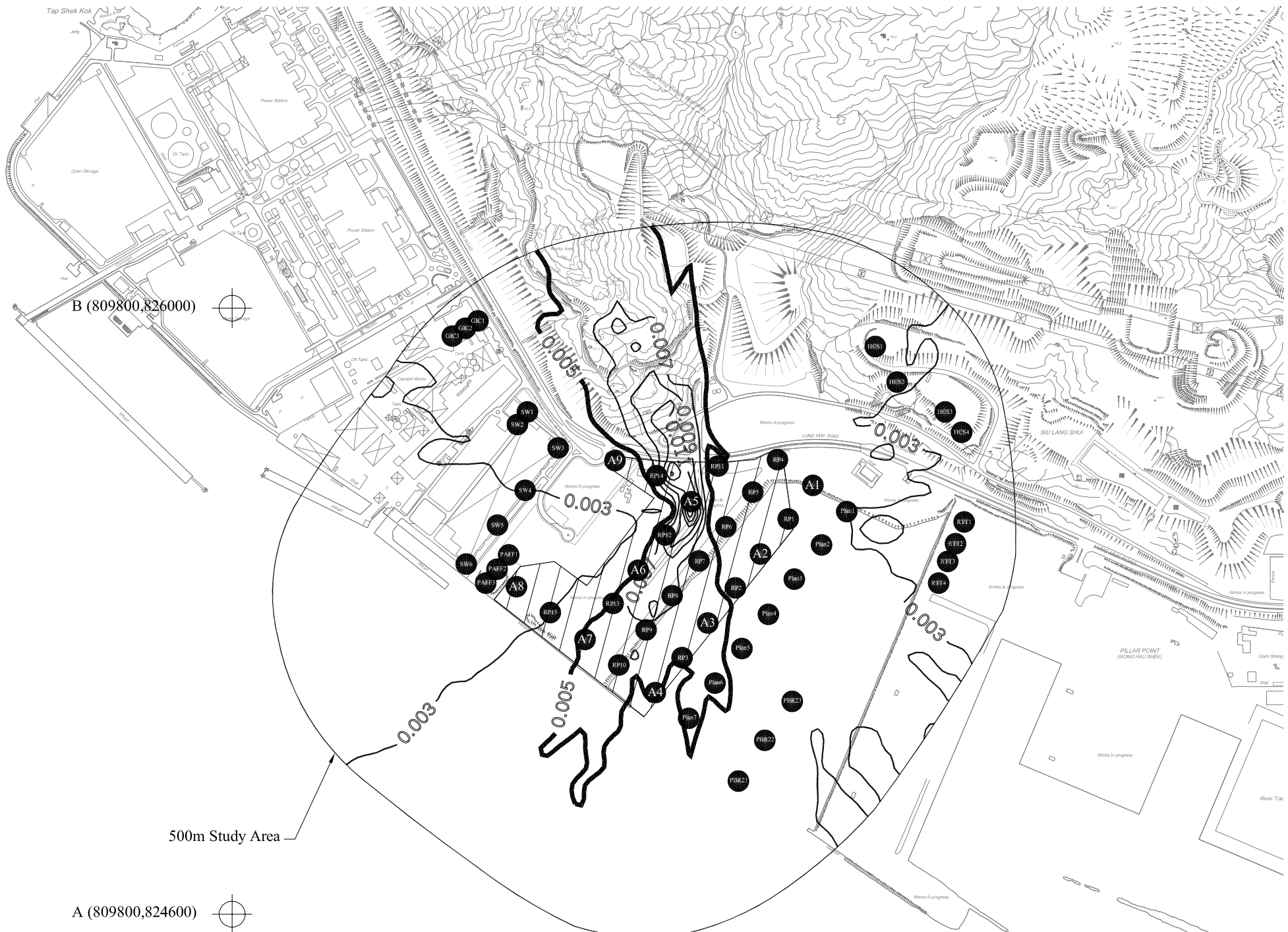
Scale: As shown Figure 7-I6 Cumulative 1-year Cd Concentration ( \mu\text{g}/\text{m}^3 ) at 61.5mPD emitted from Source Location A5 (Mitigated Scenario 2)
