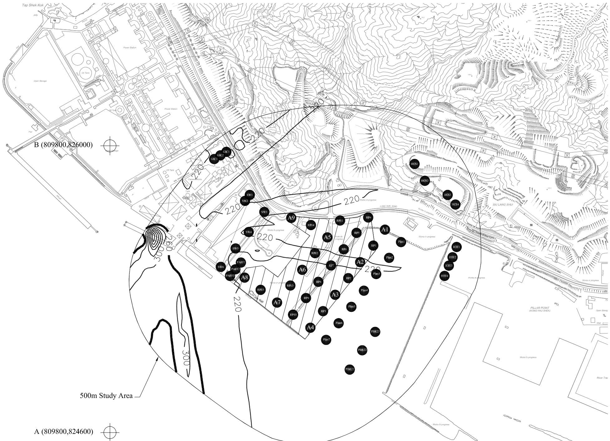
Scale: As shown Figure B8-A4 Cumulative 24-hour TSP Concentration ( \mu\text{g}/\text{m}^3 ) at 17.3mPD emitted from Source Location A3 (Scenario 3 Phase I Eco Park with CEDD Fill Bank & Other Facilities)
