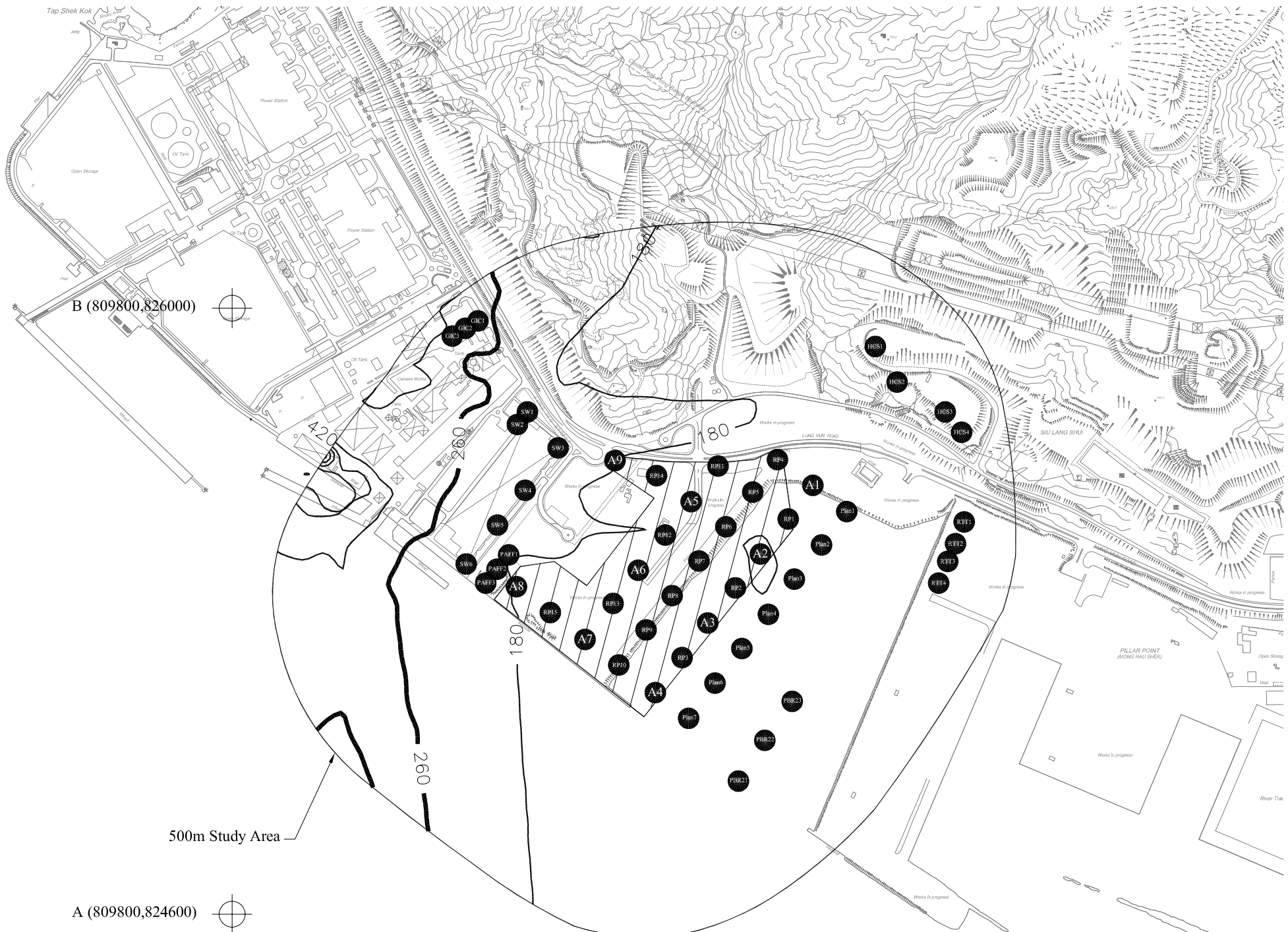
Scale: As shown Figure 8-A6 Cumulative 24-hour TSP Concentration ( \mu\text{g}/\text{m}^3 ) at 61.5mPD emitted from Source Location A2 (Scenario 3 Phase I Eco Park with CEDD Fill Bank & Other Facilities)
