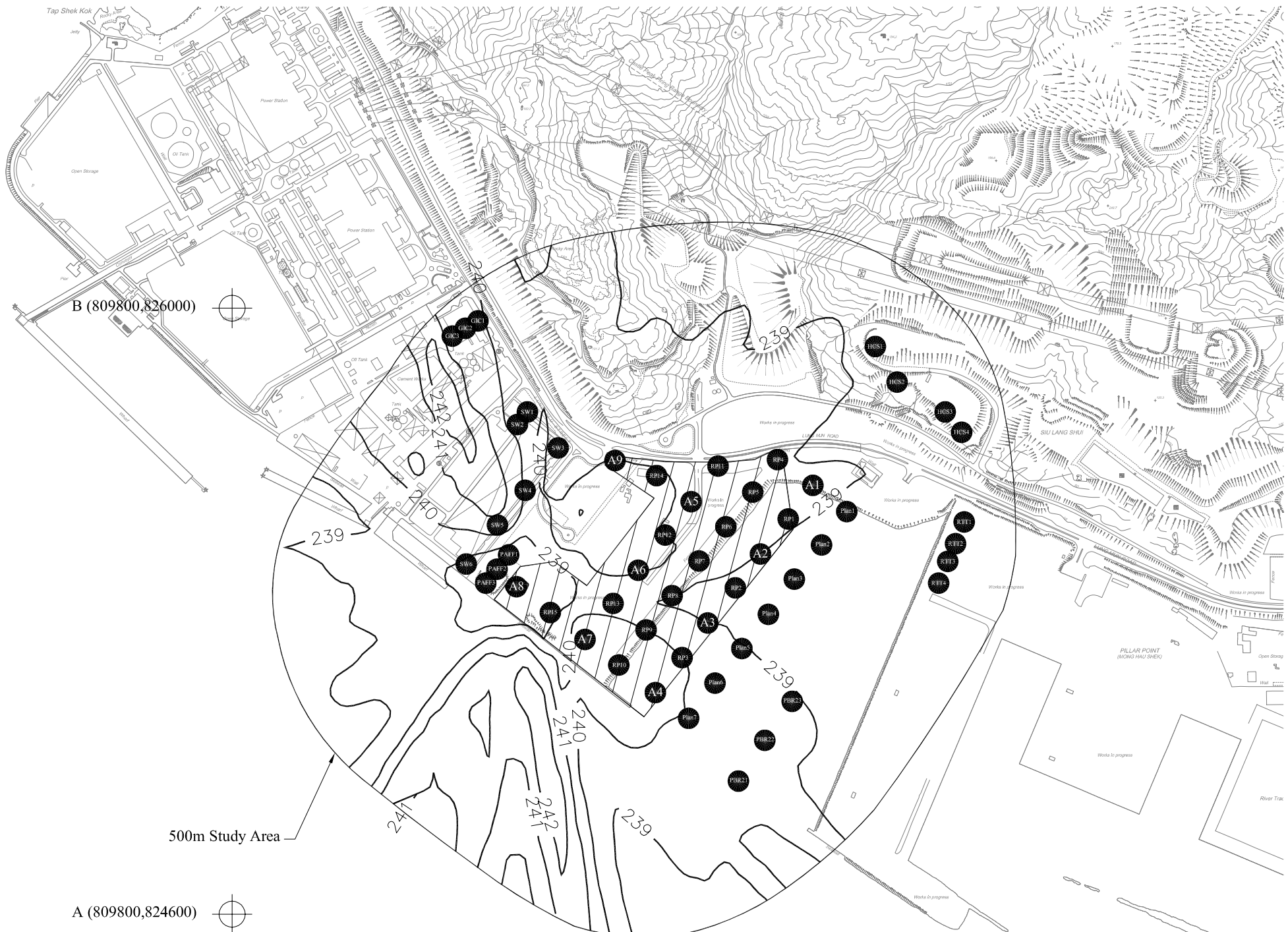
Scale: As shown Figure 8-A3 Cumulative 24-hour TSP Concentration ( \mu\text{g}/\text{m}^3 ) at 8.5mPD emitted from Source Location A8 (Scenario 3 Phase I Eco Park with CEDD Fill Bank & Other Facilities)
