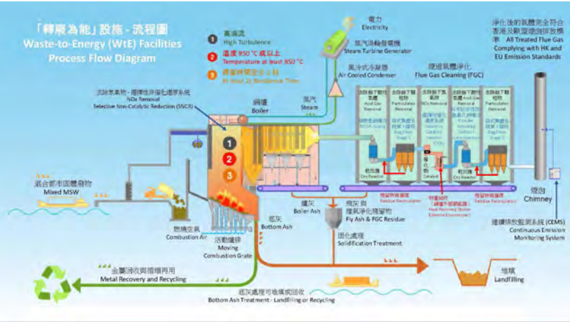
The planned MSW incineration and flue gas treatment processes of I-PARK
