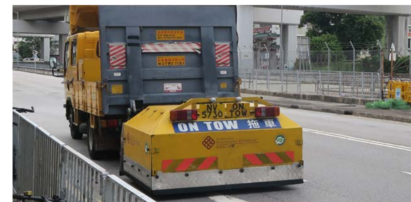
| Close-Proximity (CPX) trailer conducting road-tyre noise measurements
