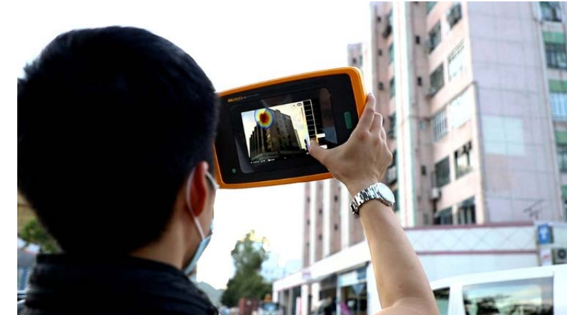
Innovative portable "acoustic camera" was mainly used in investigating commercial and industrial noise
