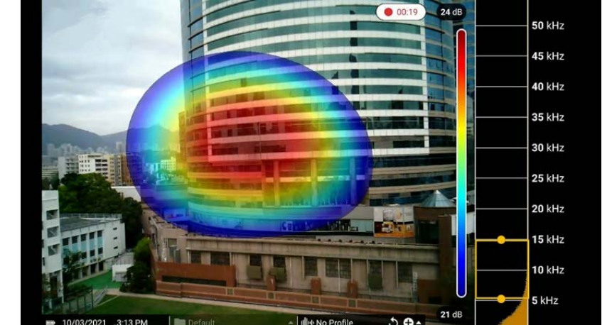
From the different colours displayed on the screen of the "acoustic camera", investigators of the EPD can "see" the location of the noisiest source at a glance
