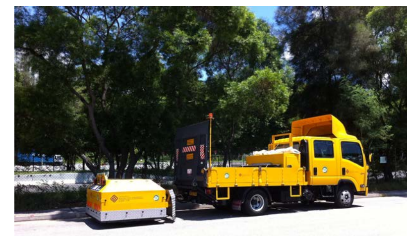
Overview of CPX trailer and towing vehicle
