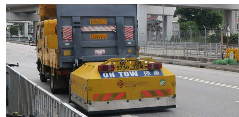
Close-Proximity (CPX) trailer conducting road-tyre noise measurements
