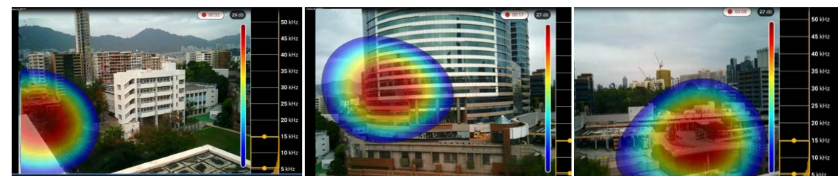
Identification of noise sources displayed on the screen of the "acoustic camera"
