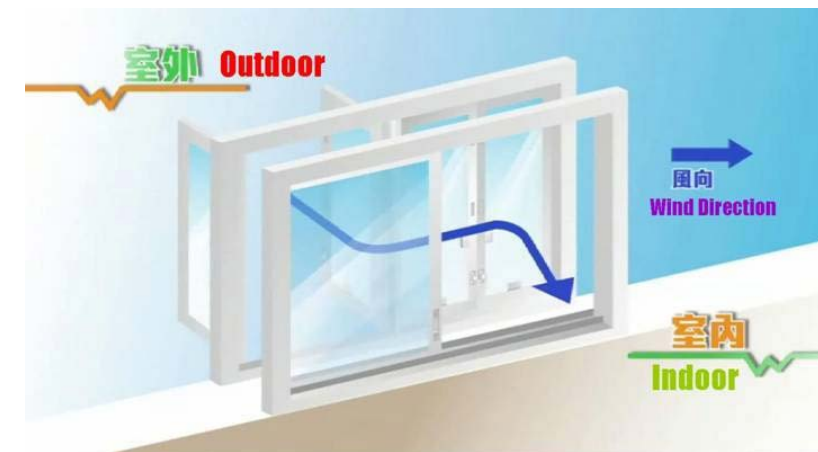
| Schematic diagram of baffle type acoustic window
